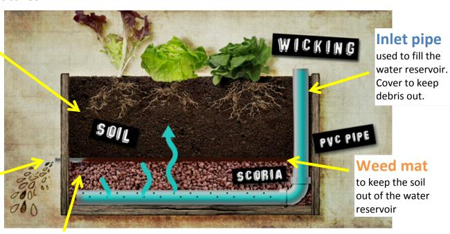
**Water reservoir** Create with pond liner or use a vessel that's watertight! Fill with scoria, sand or other inorganic media to support the soil and store the water. Depth can vary. More water held means less frequent watering. Water 'wicks' into soil.
